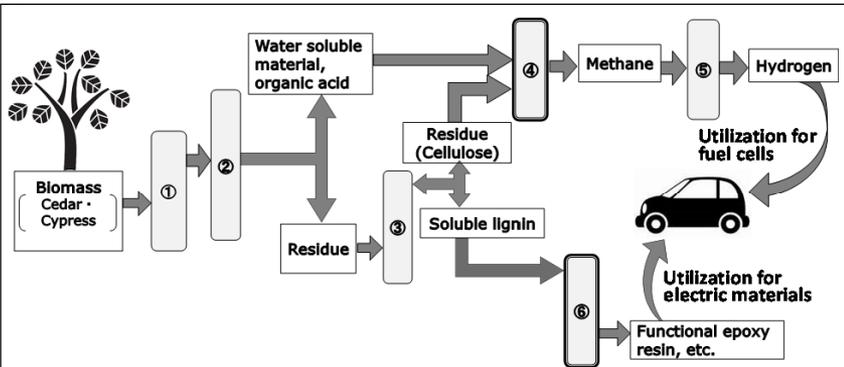
Fig.1 Collaborative creation system of hydrogen and resin from plant biomass. ① Steam explosion, ② Water extraction, ③ Acetone extraction, ④ Methane fermentation, ⑤ Steam reforming, ⑥ Resinification.
